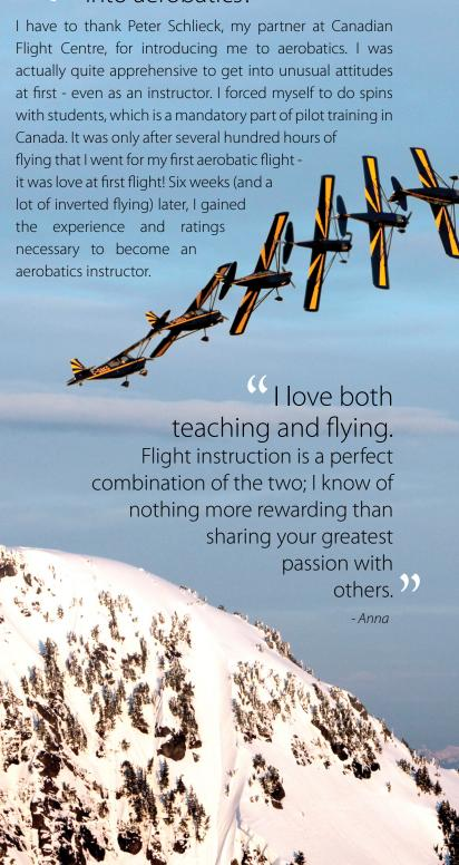
• What do you fly? My 'dancing partner' is Canadian Flight Centre's Super Decathlon, a plane built by American Champion Aircraft specifically for aerobatics training. It has inverted oil and fuel systems that allow sustained inverted flight, and is designed to withstand the severe g-forces experienced during aerobatic maneuvers. After my flight, I'd love to meet you and introduce you to the Decathlon.
